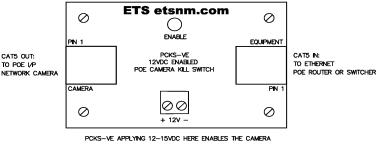
PCKS-VD APPLYING 12-15VDC HERE DISABLES THE CAMERA
