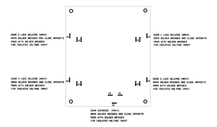
Figure 3 Configuring dry contact to isolated voltage lock control input. Bridge all "VI" contacts.
